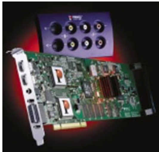
Figure 2. The Pinnacle Pro One full-slot compression board with break-out box comes with an assortment of video-editing software.
